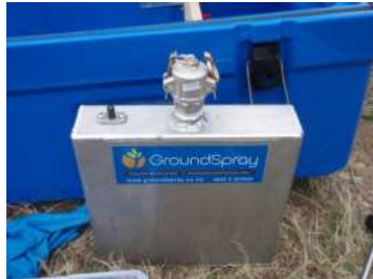
Figure 4: The components of a closed-system, 5 L electrically operated knapsack developed by Marty Grounds of Groundspray Ltd. The photograph on the right shows an example of a closed-system herbicide container used to protect operators from spillage. These knapsack systems are available from Marty Grounds (027 228 6566) for $1500 each. (Photographs: Mark Dean)
