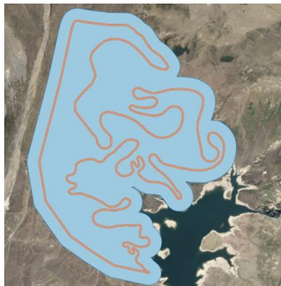
Flight Path processed into a polygon using a buffer and union tool so there are no gaps when an area is fully enclosed
