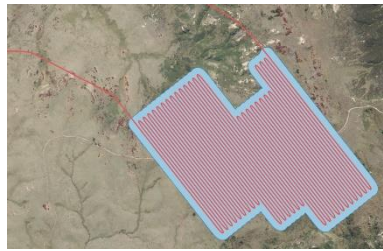
Flight Path processed into a polygon using a buffer and union tool so there are no gaps when an area is fully enclosed
